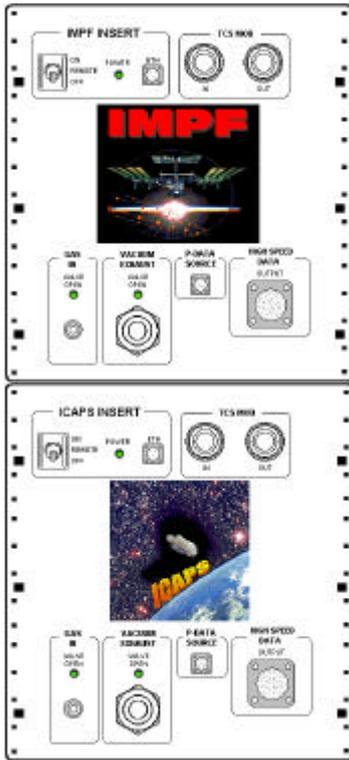
Figure 11: Standardized interfaces for IMPF and DPF Experiment inserts
