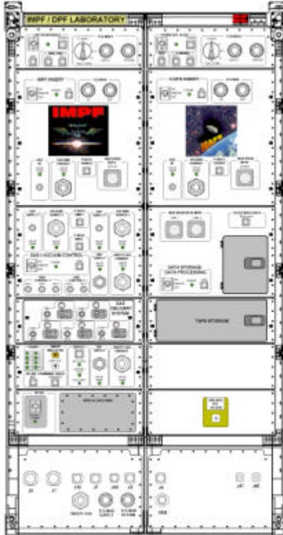
Figure 12: Accommodation layout and interfaces for IMPF/DPF Laboratory
