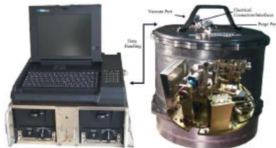
Figure 3: PKE-Nefedov Hardware: Telescience Unit and Experiment Unit [3]
